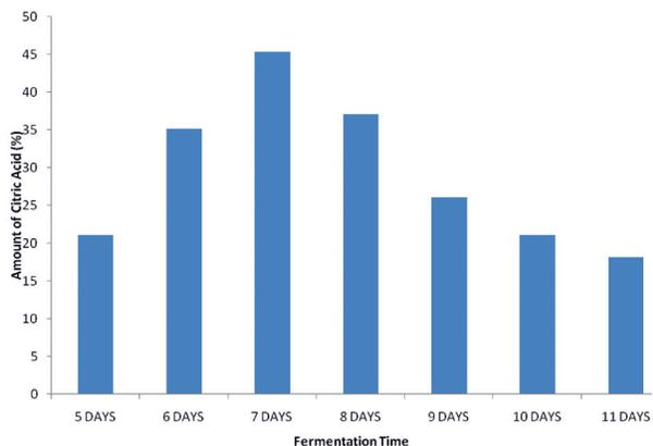
Fig. 4. Effect of Time course on Citric acid produced from ASHUS7 in a Submerged Medium.
