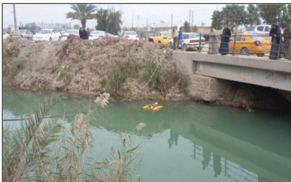
Fig. 7. Field measurement of Al-Mahawil stream using River Surveyor Tool
