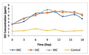
**Fig. 2.** DO concentration throughout the research after the addition of elements K and C
