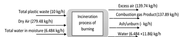
Fig. 1. The material balance scheme of design process incineration of unusable plastic
